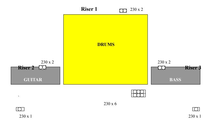
(W x D x H) **Riser 1** ------ 2,5m x 2,5m x 0,4m **Riser 2 & Riser 3** ----- 1,0m x 0,5m x 0,4m
